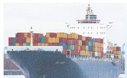
Largest container vessel to date MSC Ningbo Adelaide16/12/2016 L:300m B: 42.86 GRT: 83,133 7,849TEU 17 containers across deck
