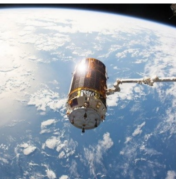
The Japanese HTV-6 cargo craft in the grip of a Canadian Space Agency robotic arm after it was detached from the Harmony module of the International Space Station.
