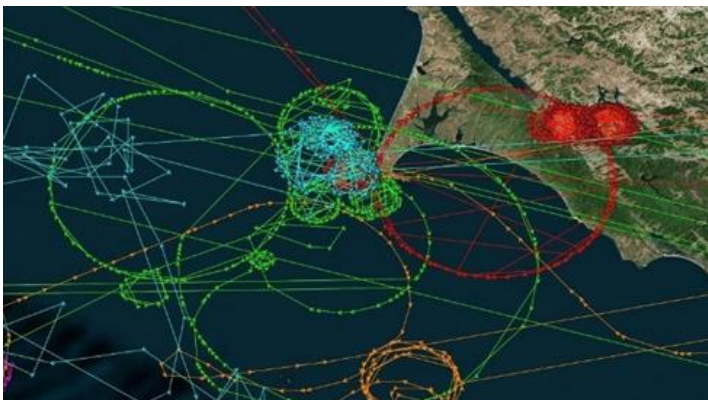
Erroneous AIS data purporting to show the "positions" of vessels affected by GPS spoofing (Illustration courtesy Skytruth)
